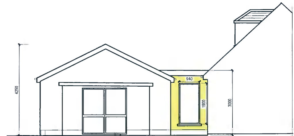
SIDE ELEVATION (WEST) - INTER CONNECTING LOBBY
