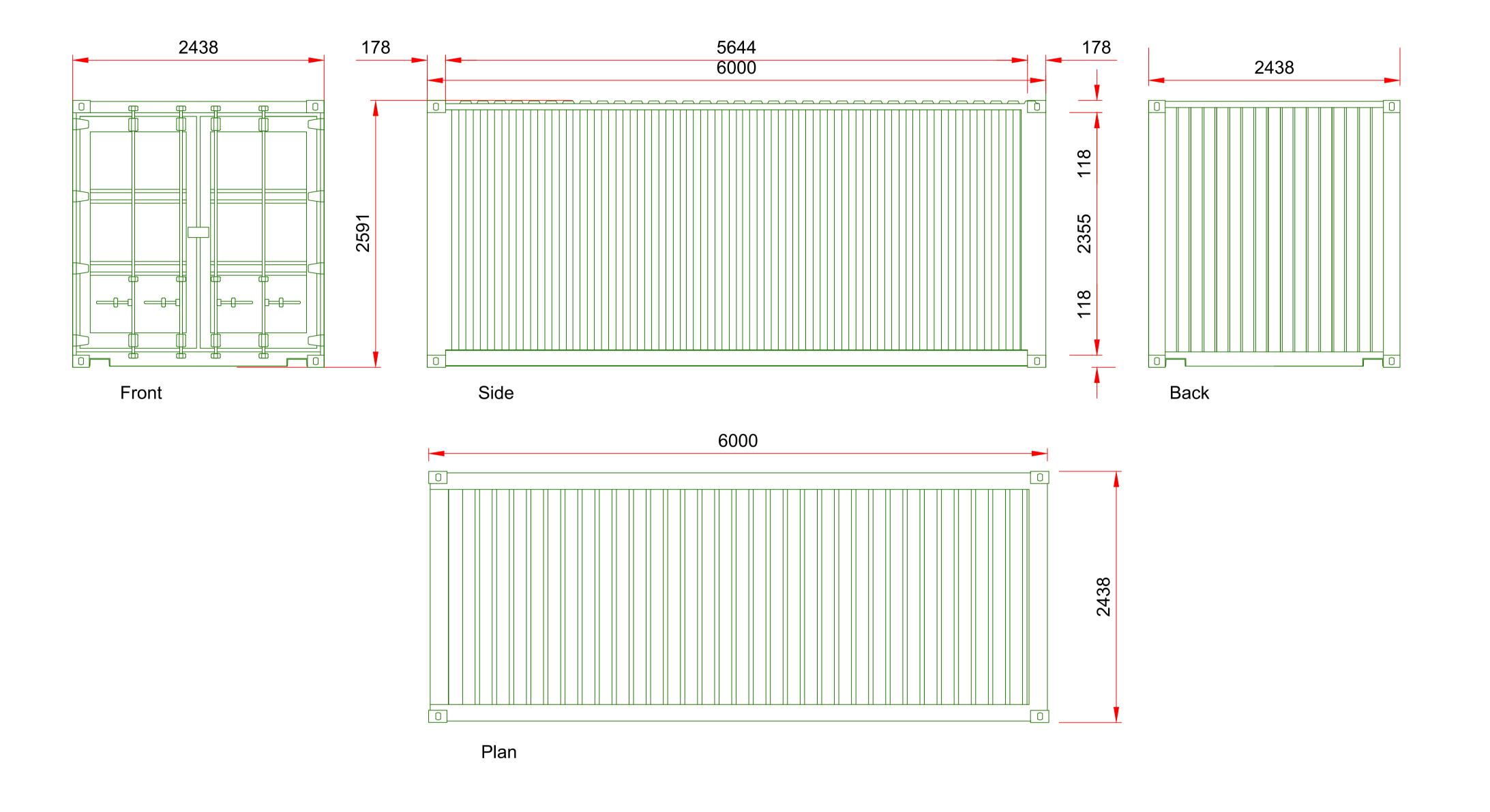
STEEL STORAGE CONTAINER ELEVATIONS AND PLAN
