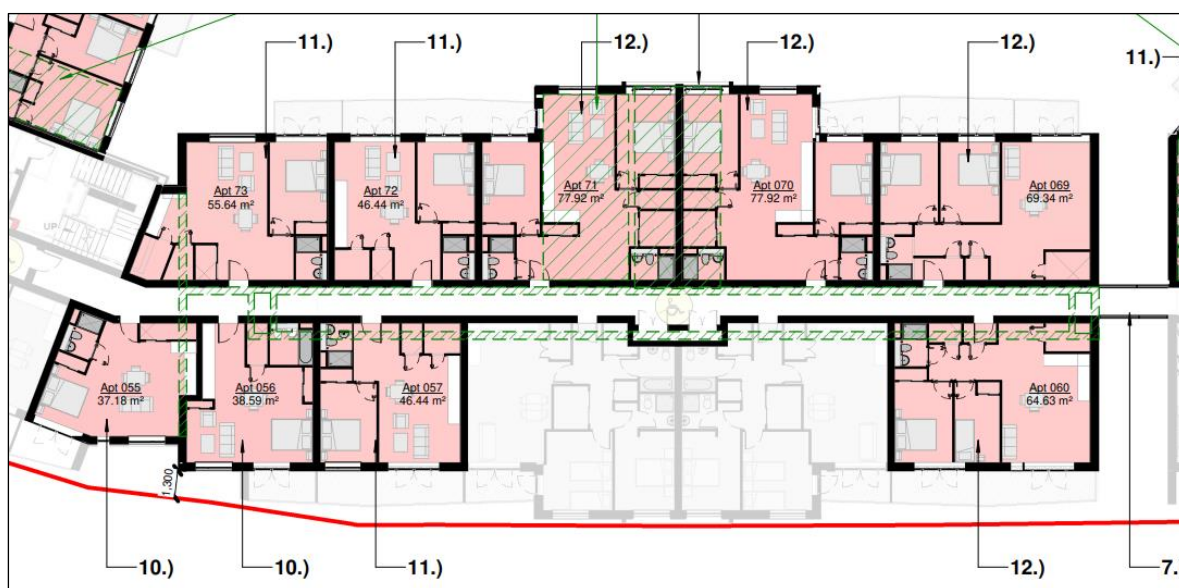
Figure 33.0 Excerpt from first floor plan of development proposed under S146B amendment illustrating revised apartment configuration proposed in Block C
