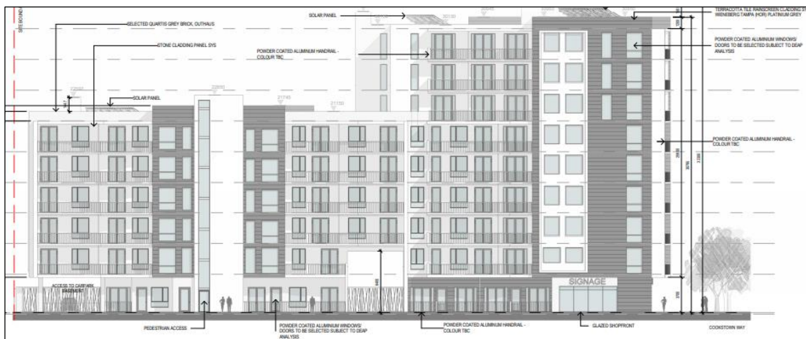
Figure 14.0 Northern elevation (fronting onto Second Avenue) of development approved under ABP Ref. 303803-19
