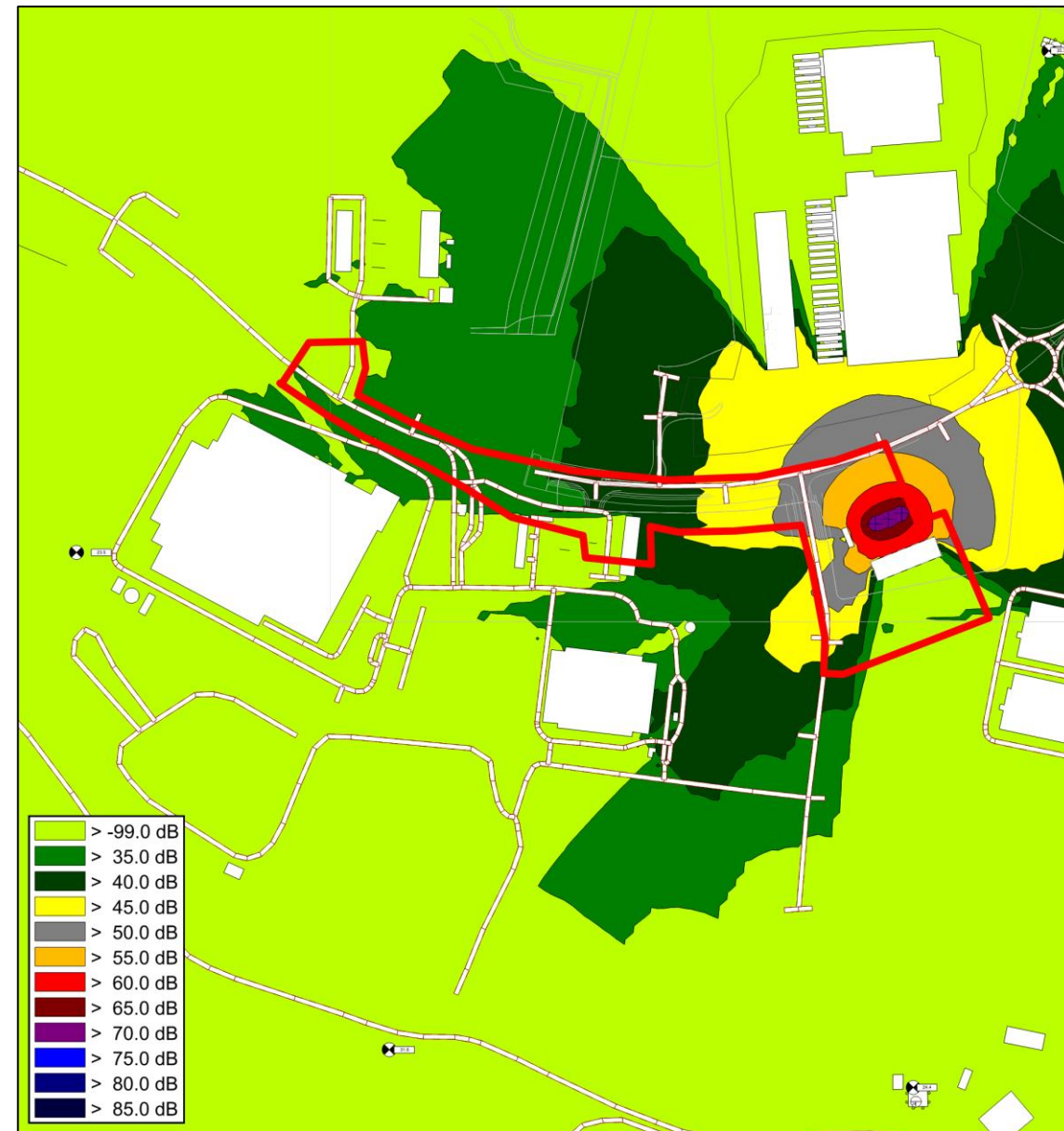
Figure 9.5: Overview of Modelled Noise Emissions (dBA during daytime and night time - grid set at 4.0AGL)
