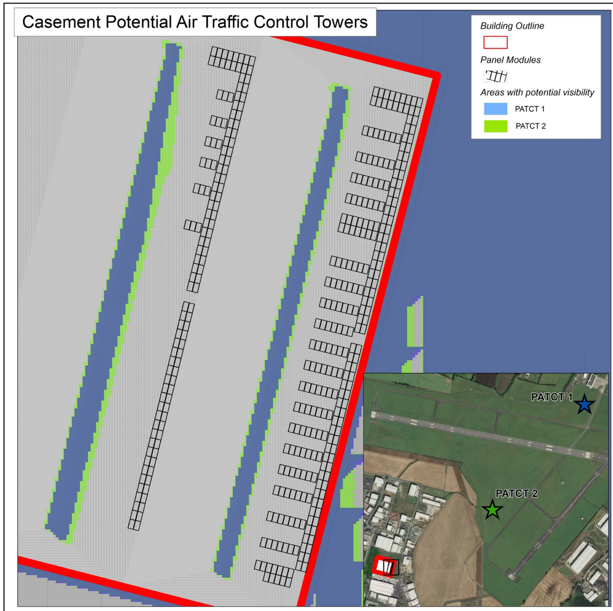
Figure 12: Output of results of ZTV analysis showing areas that are theoretically visible from the future potential ATCT at Casement Aerodrome.
