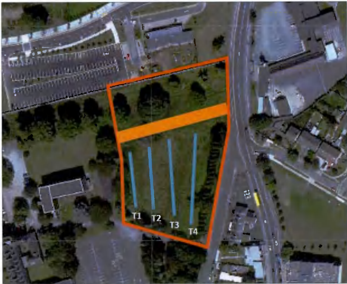
Figure 8: Location of excavated test trenches (Source: https://maps.archaeology.ie/HistoricEnvironment/ ) The location of an existing gas pipeline is marked by orange line
