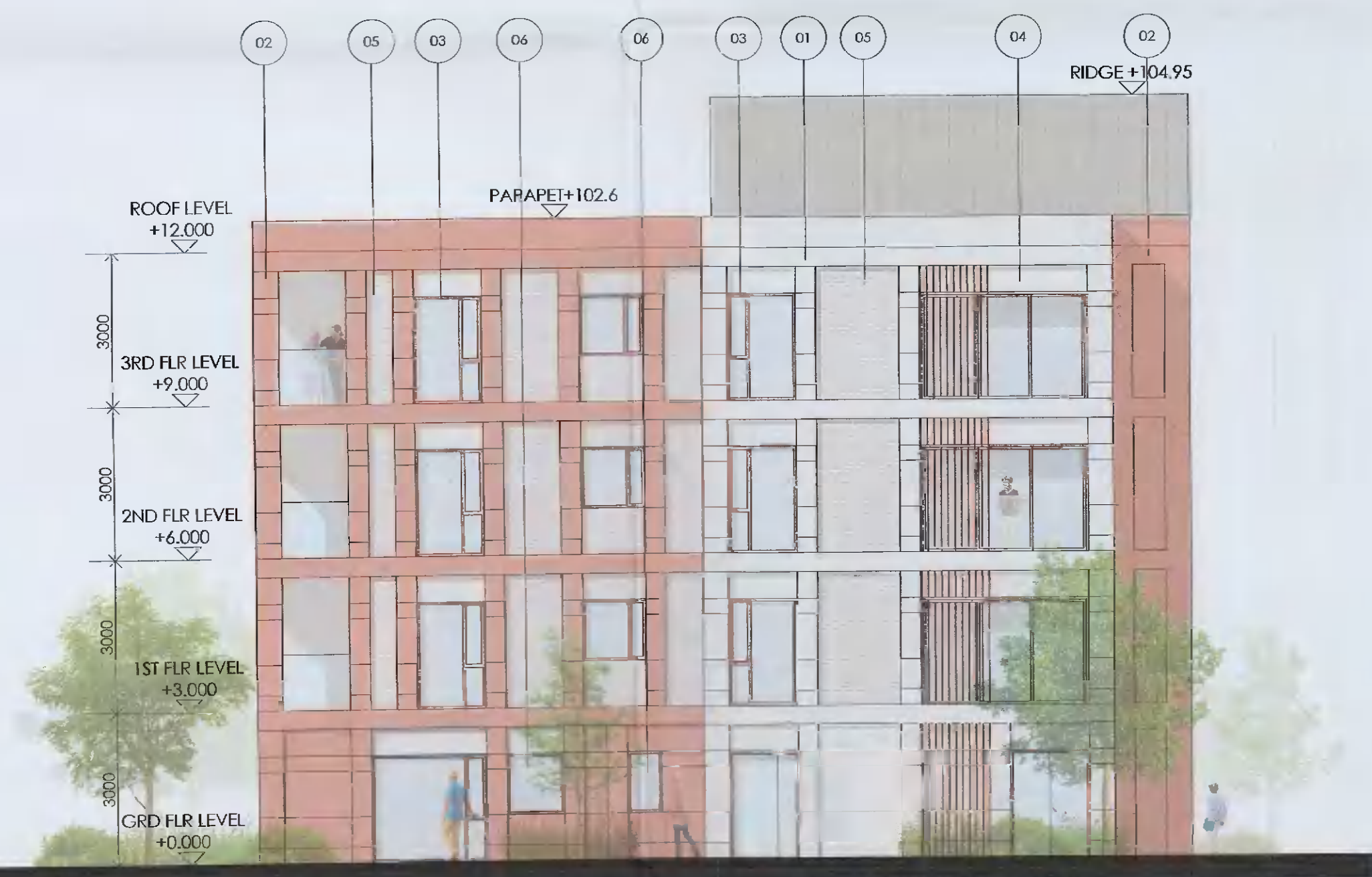
BLOCK A SOUTH ELEVATION SCALE 1:100
