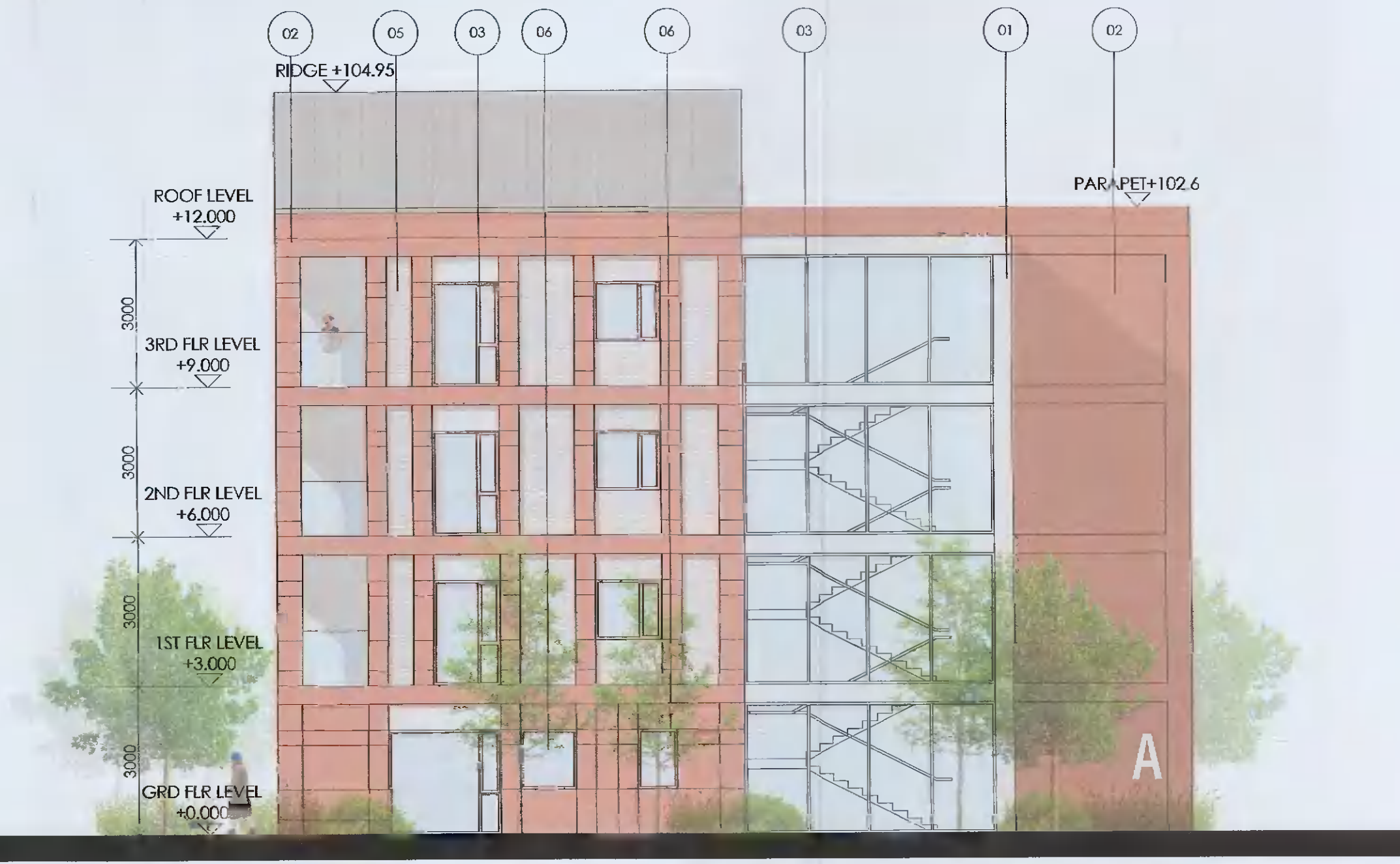
BLOCK A NORTH ELEVATION SCALE 1:100
