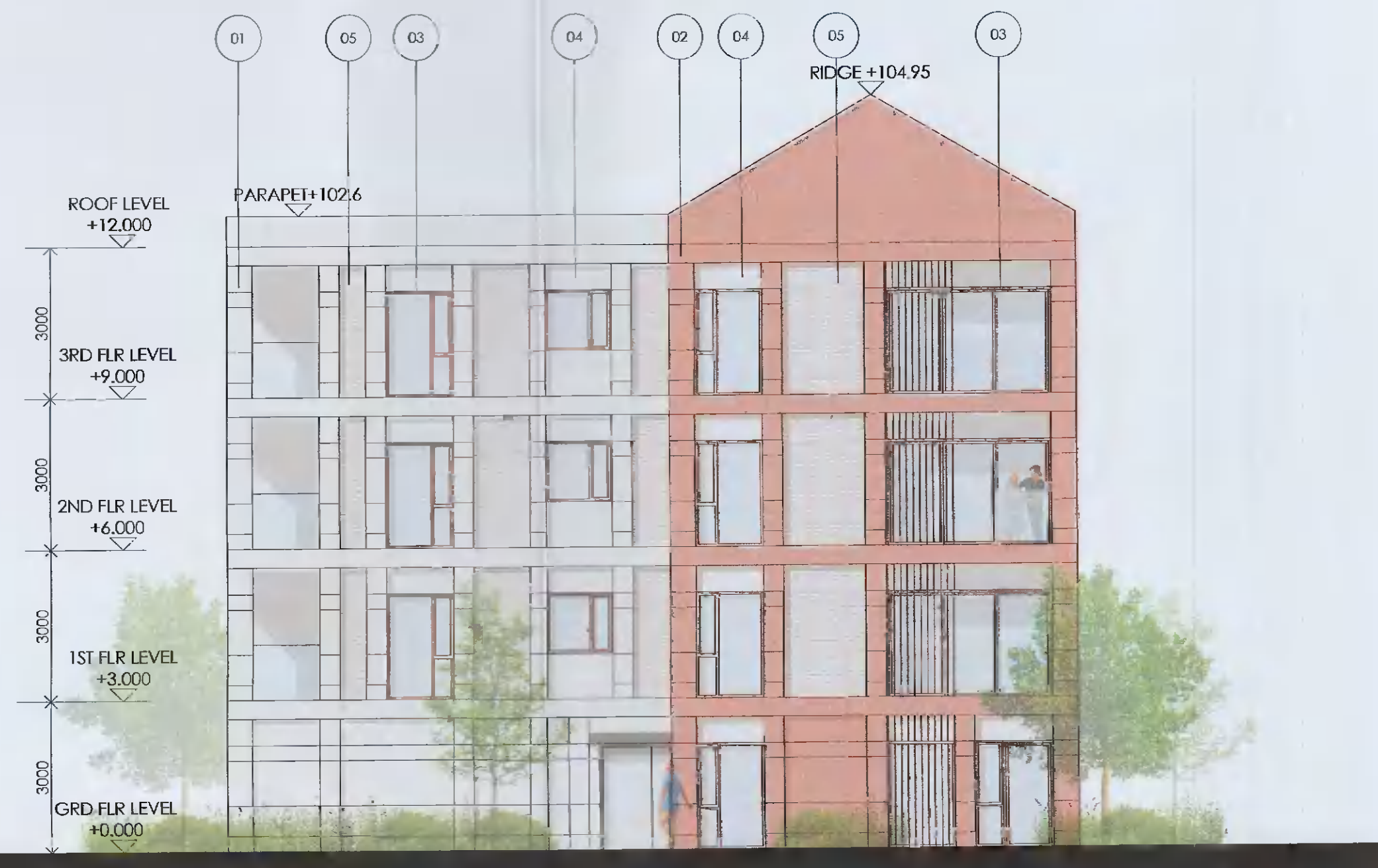
BLOCK A EAST ELEVATION SCALE 1:100
