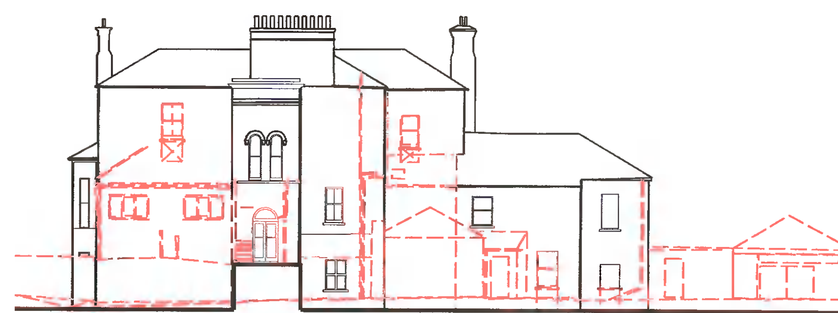
DEMOLITION - ELEVATION TO SOUTH - 1:200
