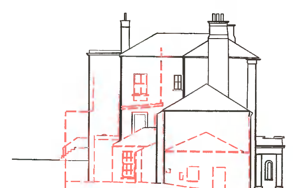
DEMOLITION - ELEVATION TO WEST - 1:200
