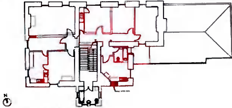
DEMOLITION PLAN SECOND FLOOR LAYOUT 1:200 @ A3
