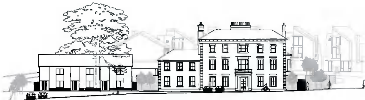
Fig. 4. Proposed Revision – integrity of front façade of protected structure retained, stone wall enclosing common gardens frames and separates the protected structure from proposed terrace which is smaller in scale and more sympathetic in form, elevational composition, and materiality to the protected structure.
