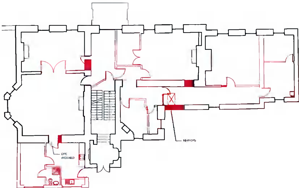
Fig. 7. – Permitted Development – first floor demolition
