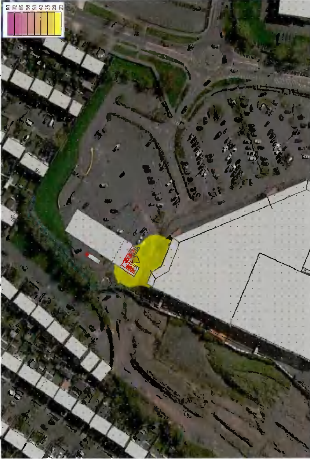
Figure 5 Night time noise contours from modelling of the roof mounted plant for the proposed development
