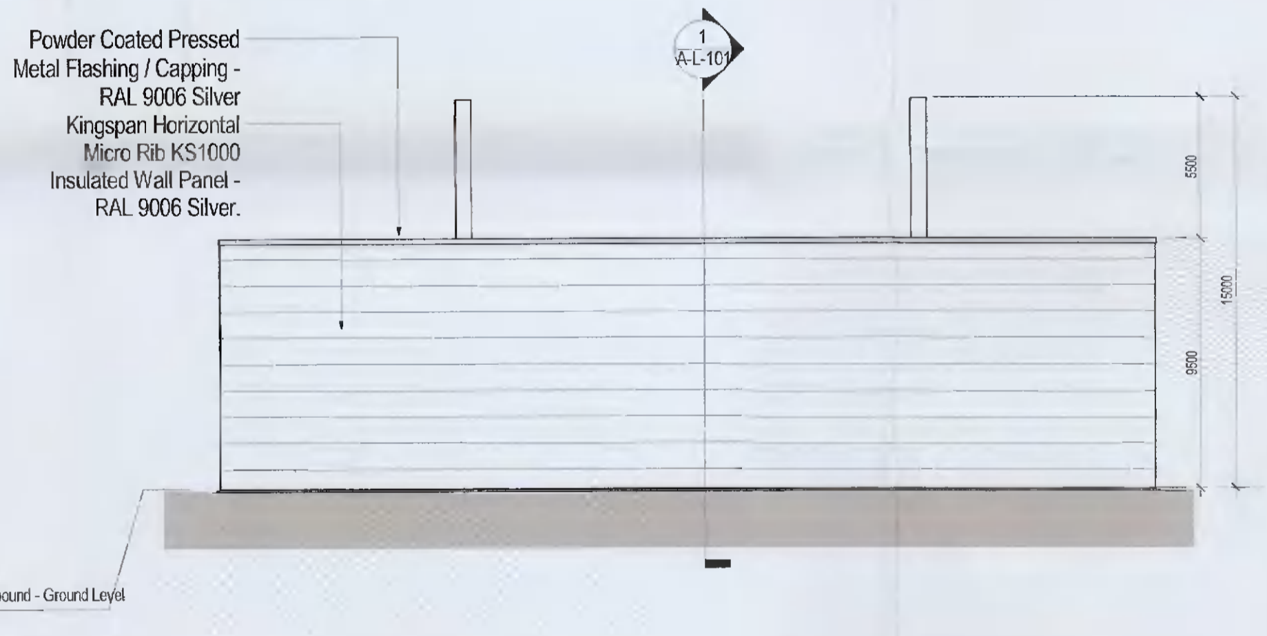
5 South Gas Generator Elevation 04 SCALE: 1:200
