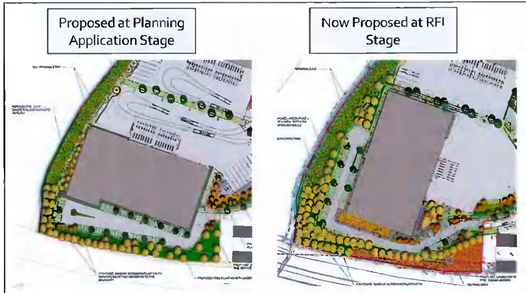
Figure 1.2.: Landscape Masterplan Proposed at Planning Application Stage (Left) and Landscape Masterplan Now Proposed at RFI Stage (Right) Showing Increased Landscape Zones and Planting to Western and Southern Boundaries.
