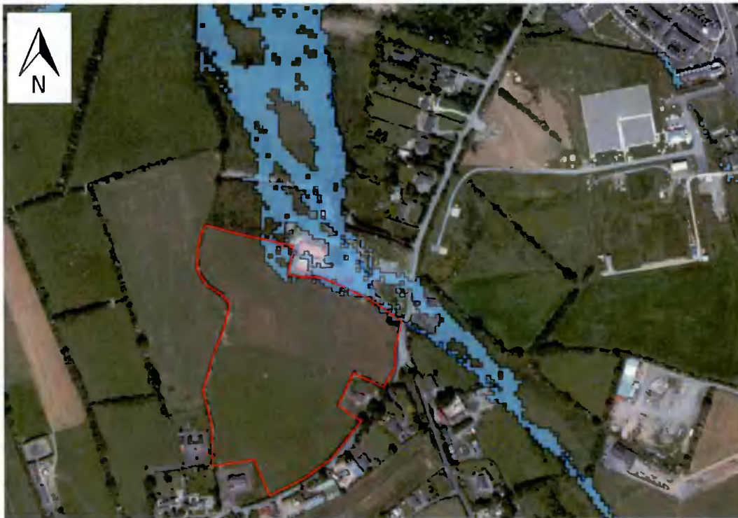
Plate 4. Extract from the Eastern CFRAM flood mapping showing the 1% fluvial flood extents based on current day scenario (i.e. site boundary outlined by red polyline).
