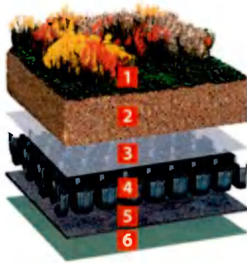
Figure 9 - Typical Extensive Green Roof
