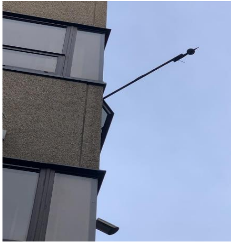
Fig 2: NML1 Mic out through window
