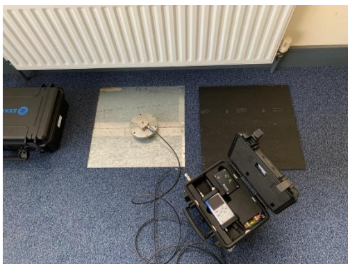
Figure 6: SVC958A in Room C.2.05 Fig 7: Direction of Triaxial Acc. on plate
