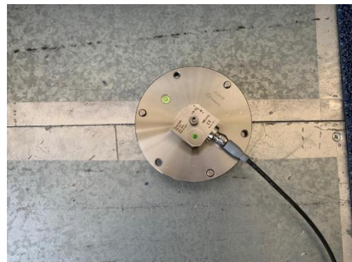
Figure 6: SVC958A in Room C.2.05 Fig 7: Direction of Triaxial Acc. on plate
