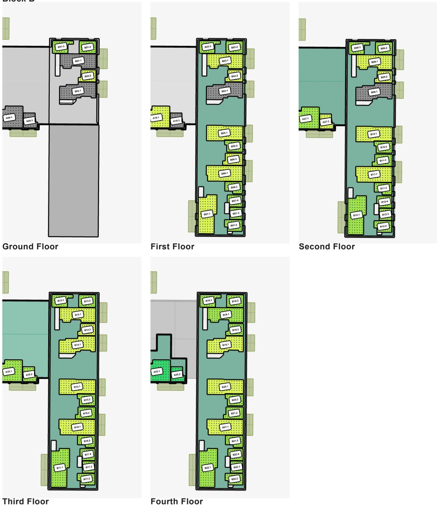
Figure 32: Block B - Daylight provision per floor.
