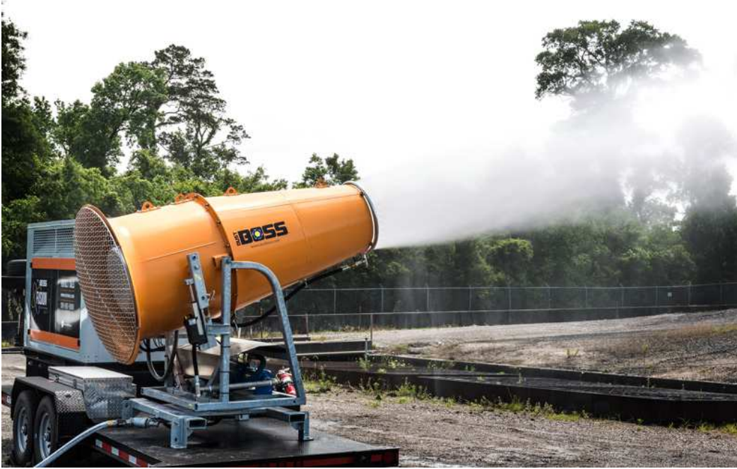
Figure 16 - Dust Suppression System
