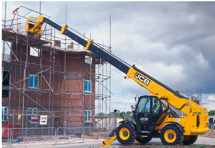
Figure 7: typical telehandler for high reach access, potentially suitable for façade panel removals
