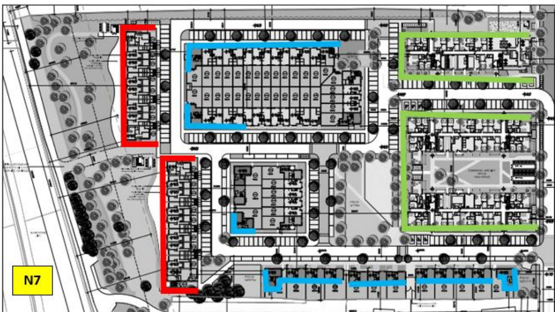
Figure 11 Mark-up of facades that require a minimum sound insulation specification on building elements.
