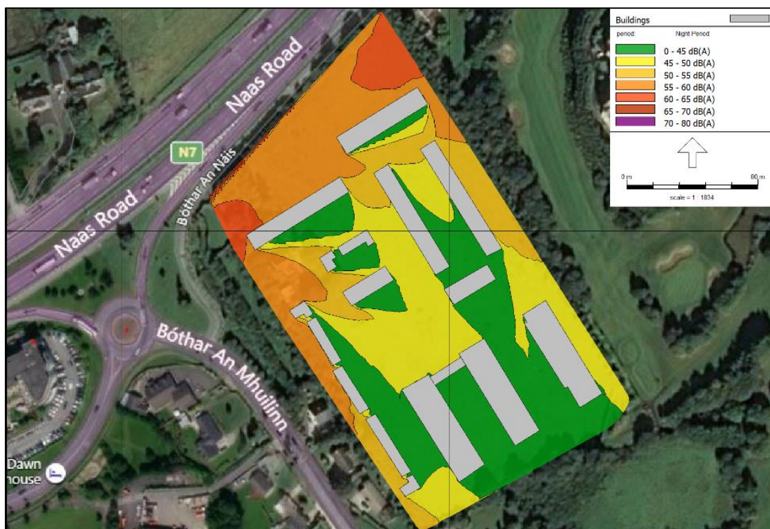
Figure 12 Amenity Noise levels Across the Development Site dB L_{Aeq,16-hour} at 1.5m height.
