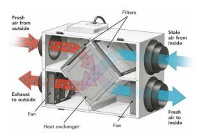
in heat losses due to ventilation is significant and occupants' comfort is also increased as the air supply is warmed before entering the rooms. The MVHR unit which houses the heat exchanger and the fans is also equipped with filters which prevent outside dust entering the system and internal air particles depositing within the unit.
