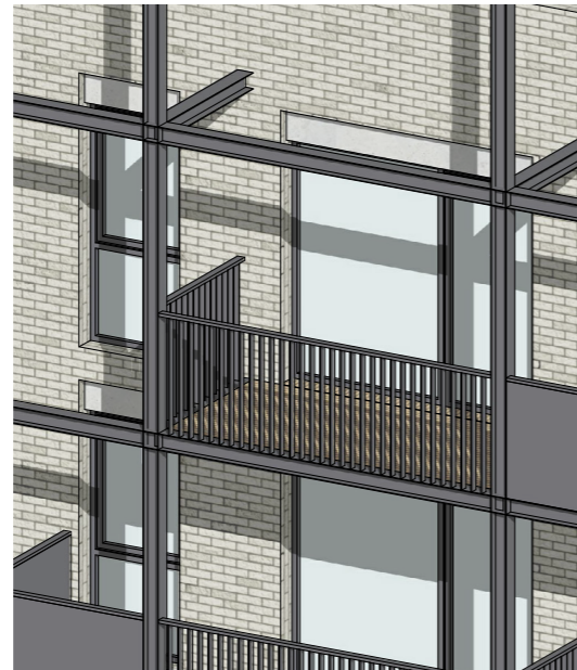
▲ CGI of study model for projecting balcony & metal balustrade supported by framed steel structure to selected colour
