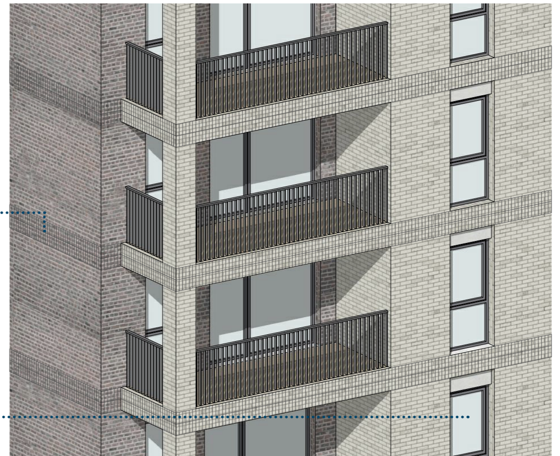
▲ Isometric View from 3D study model of typical corner balcony showing continuation of brickwork banding
