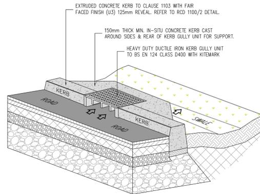
LATERAL INLET KERB GULLY SCHEMATIC.
