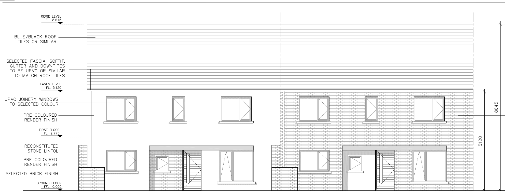
01 Alternative Elevation for Unit No's; 2,3,10,11 PA-102
