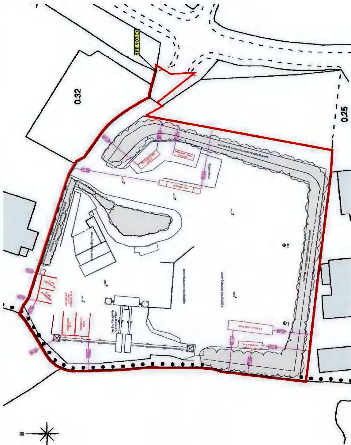
FIGURE 3. PROPOSED SITE LAYOUT (EXTRACTED FROM KILSARAN SITE LAYOUT DRAWING, DRG. NO KC02).
