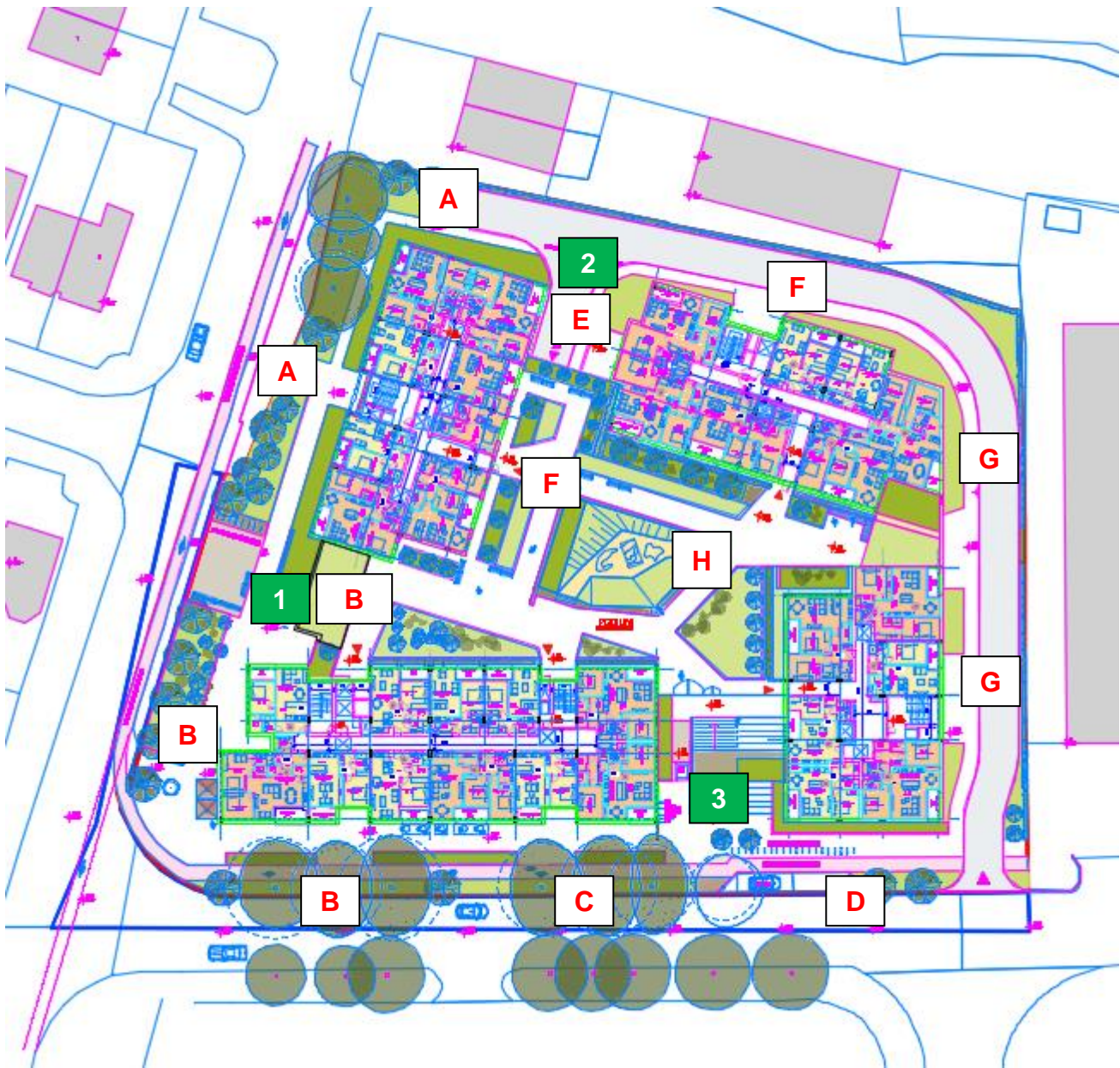
Illustration 5.3 New proposed development noise façade ID points A to G and vegetation noise barriers 1, 2 and 3 locations.
