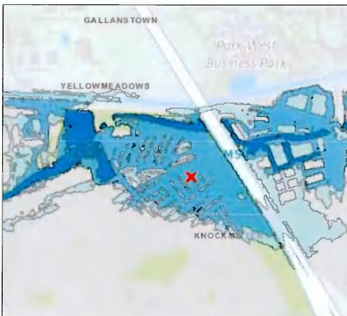
Plate 3.4: OPW mapping of fluvial extents with a mid-range future climate change allowance
