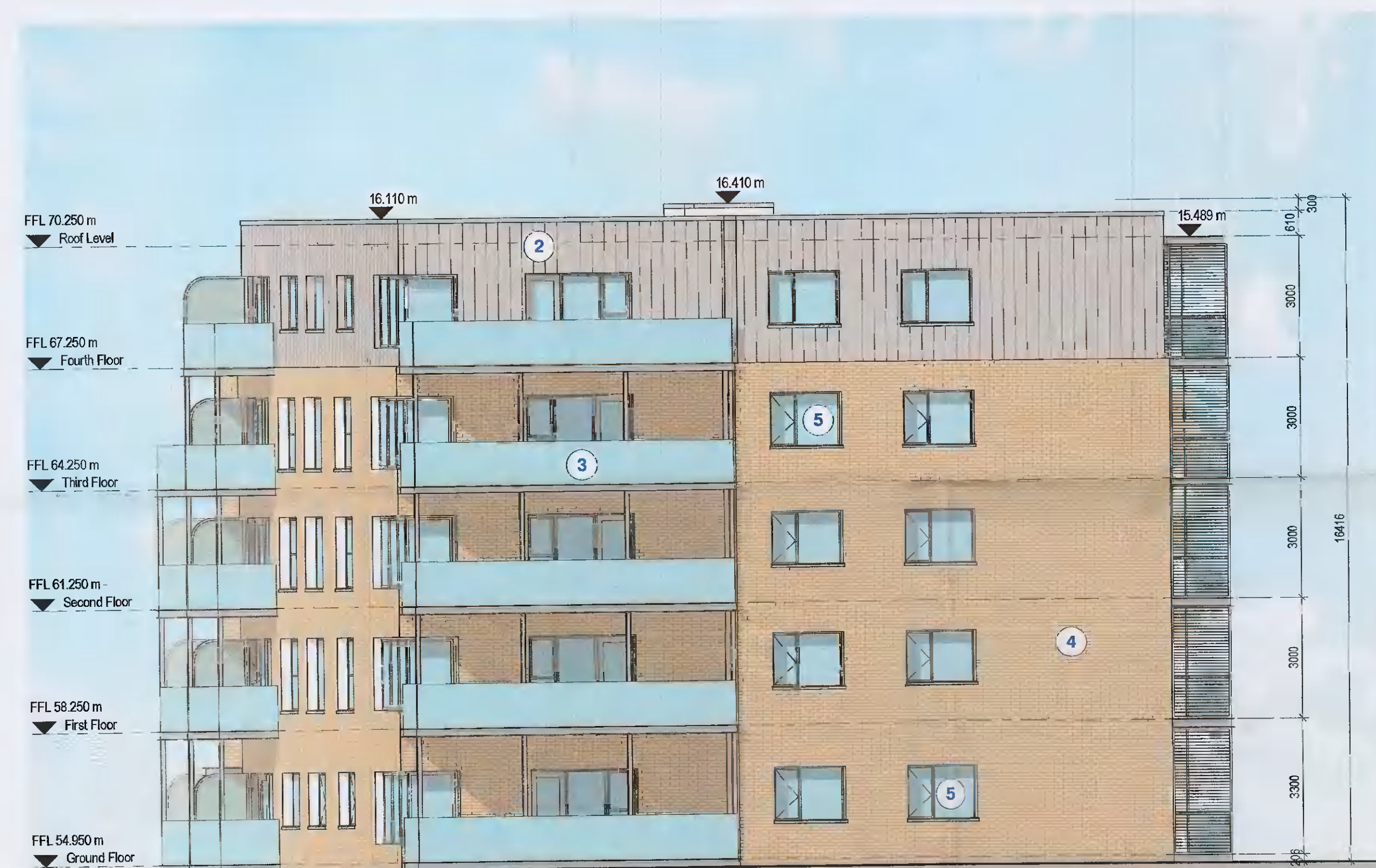
BLOCK 2 SIDE ELEVATION (EAST) 1 : 100
