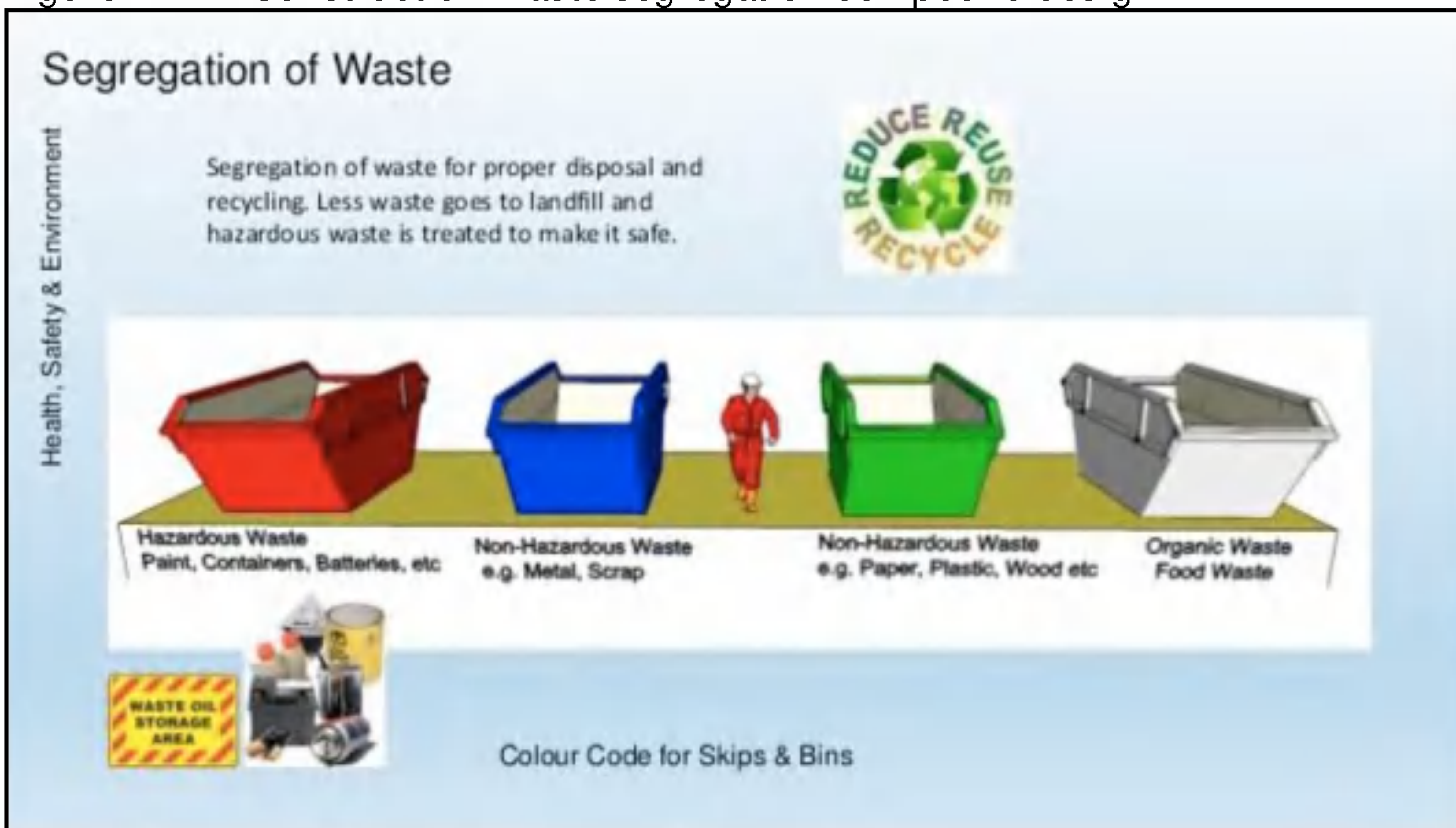
Figure 2 Construction Waste segregation compound design
