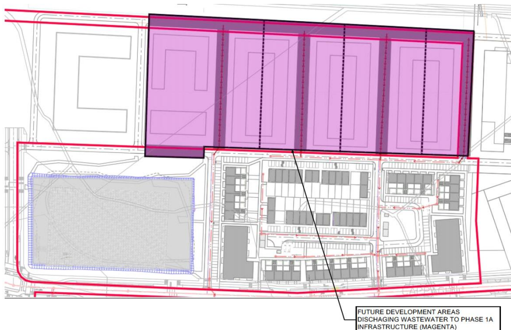
Figure 4-2 Foul Network Allowance for Future Development
