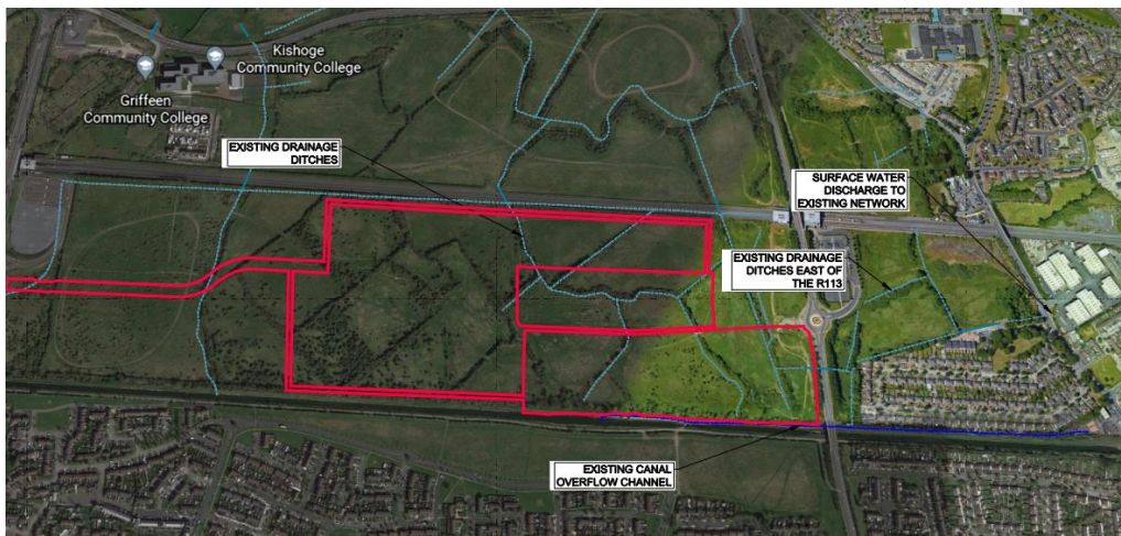
Figure 3-1 Existing Drainage (Boundary Indicative)
