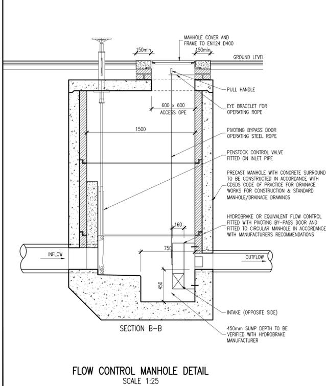
FLOW CONTROL MANHOLE DETAIL
