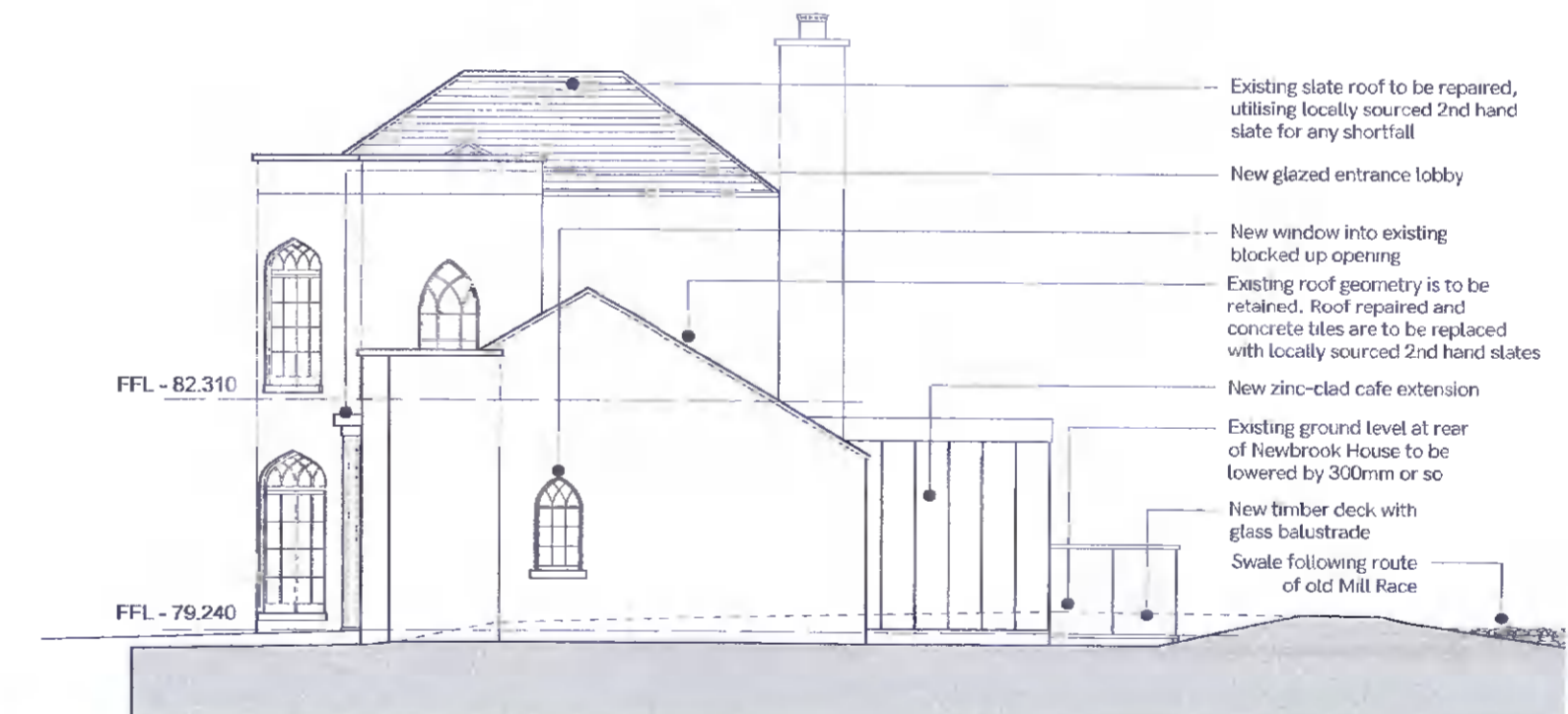
07 Existing West Elevation 1:100
