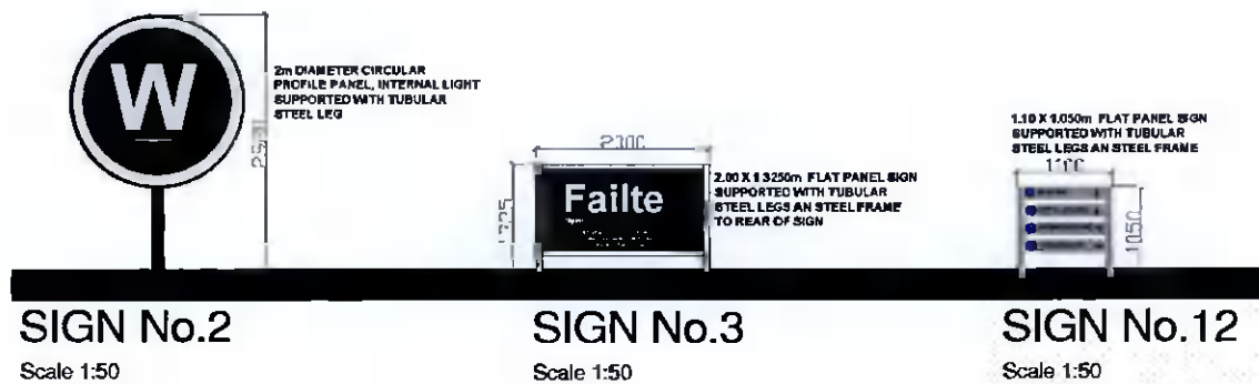
Fig A1 – excerpt from Clarke Engineers Drawing 4996-02-P1001 showing details of the signs
