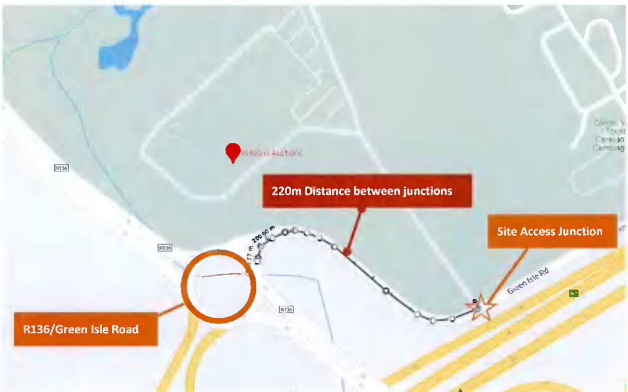
Figure 2.1: Site Access Junction Location
