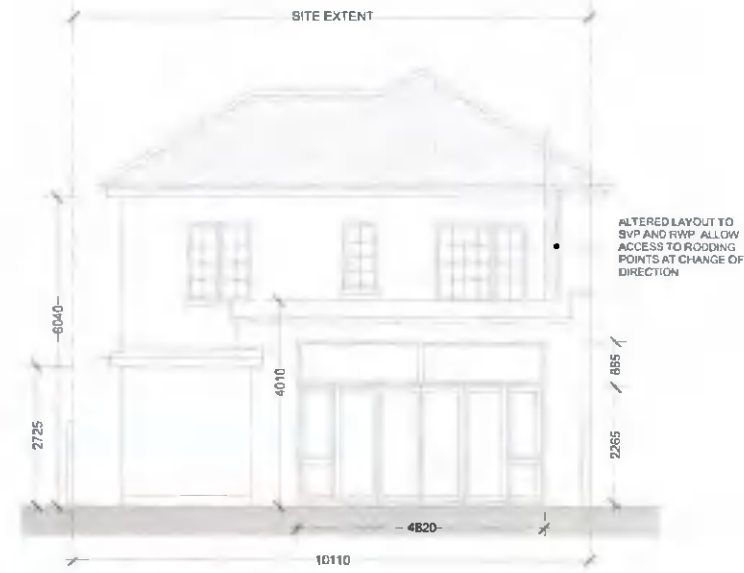
PROPOSED REAR ELEVATION SCALE 1:100@A3
