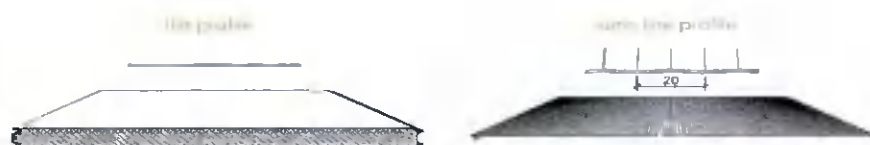
Picture 44: Composite cladding features flat for the proposed building satin line (also called micro ribbed) for the generator's enclosure.
