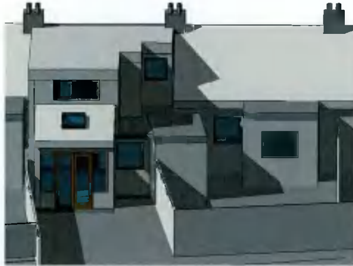
Image 2. 3D Revised design in response to FI received 14/09/21 - shadows cast midday 22 September.
