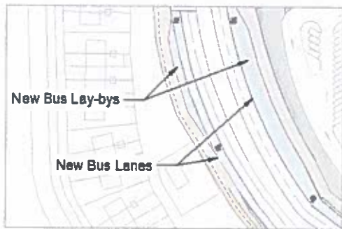
Figure 6. Planning Layout – Inset Layby's (South)
