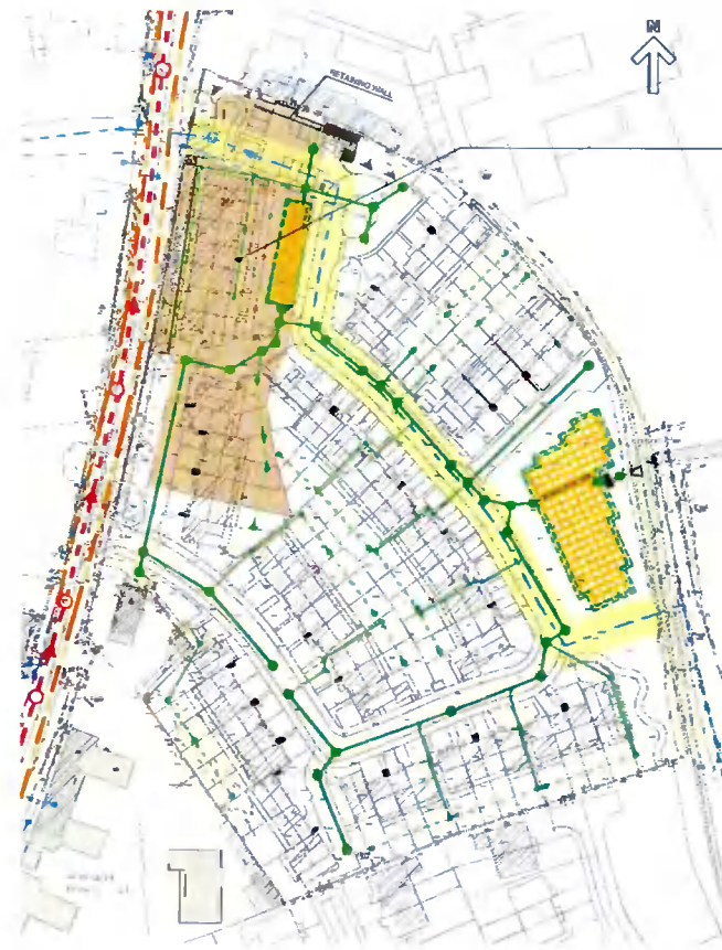
Figure 7: Plan showing extent of Ground levels to be raised to allow Surface Water to Discharge by Gravity
