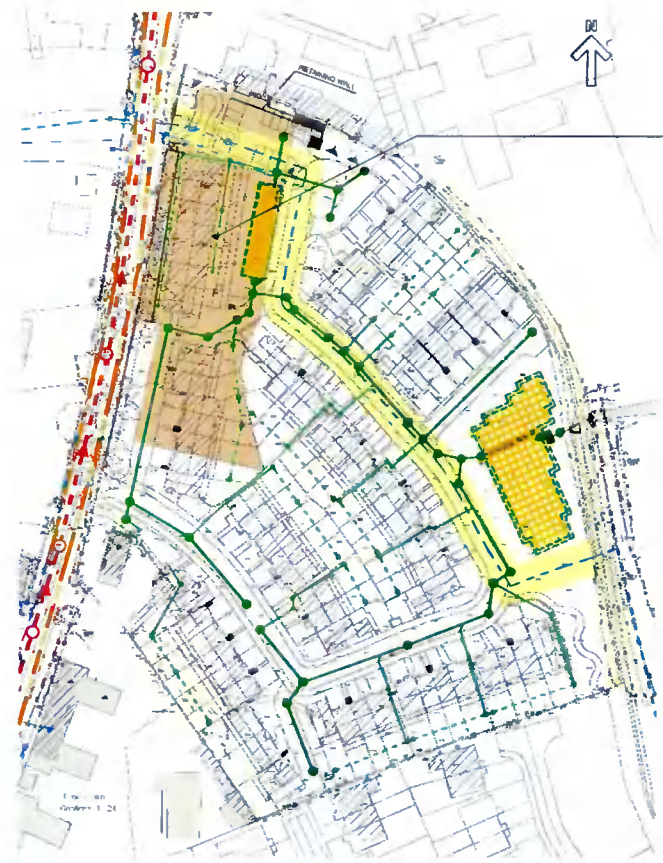
Figure 3: Site Plan Showing Extent of ground levels to be raised to achieve surface water outfall by gravity.
