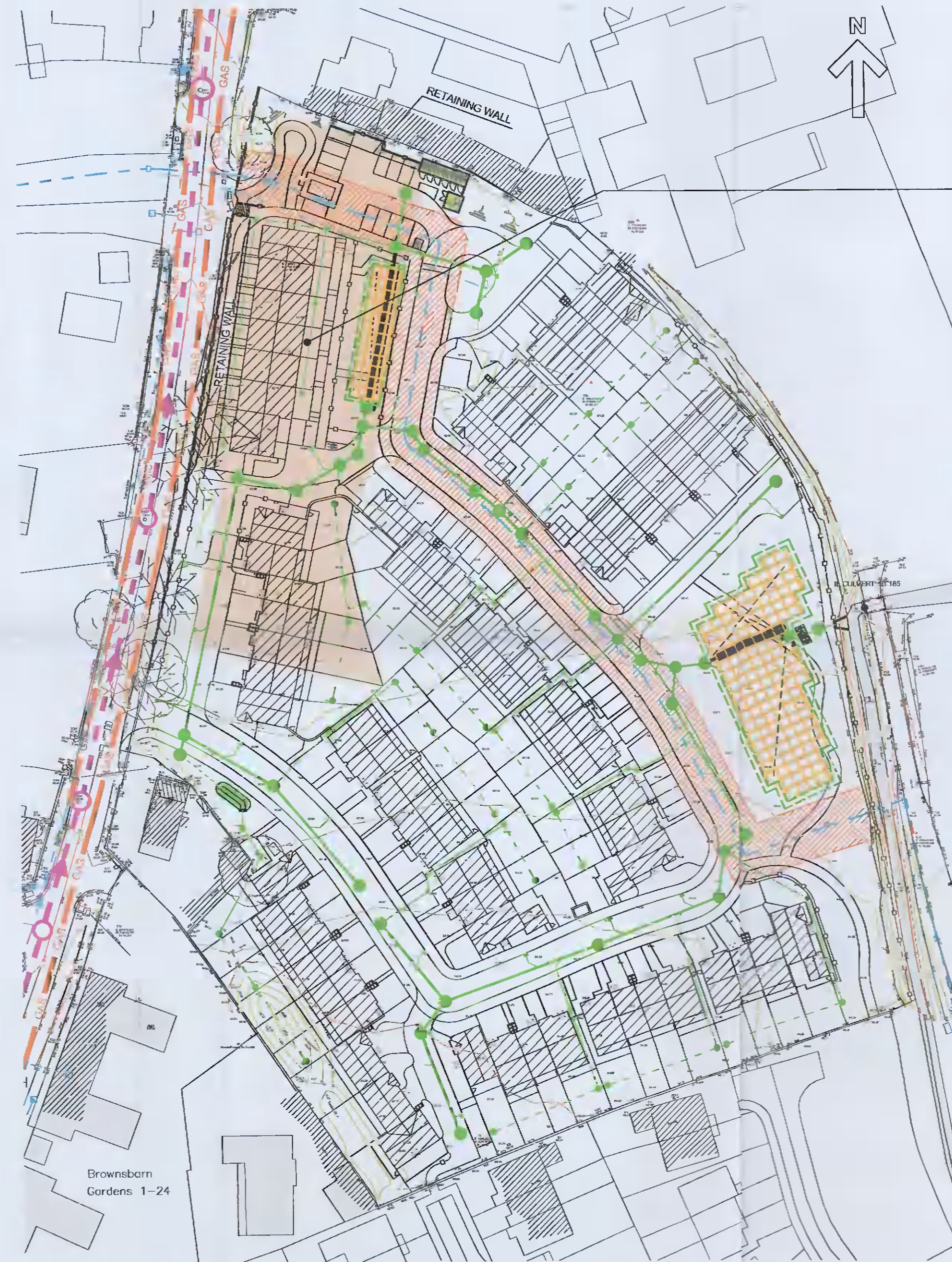
2 0054 GROUND LEVELS TO BE RAISED TO ACHIEVE SURFACE WATER OUTFALL BY GRAVITY SCALE: 1:750
