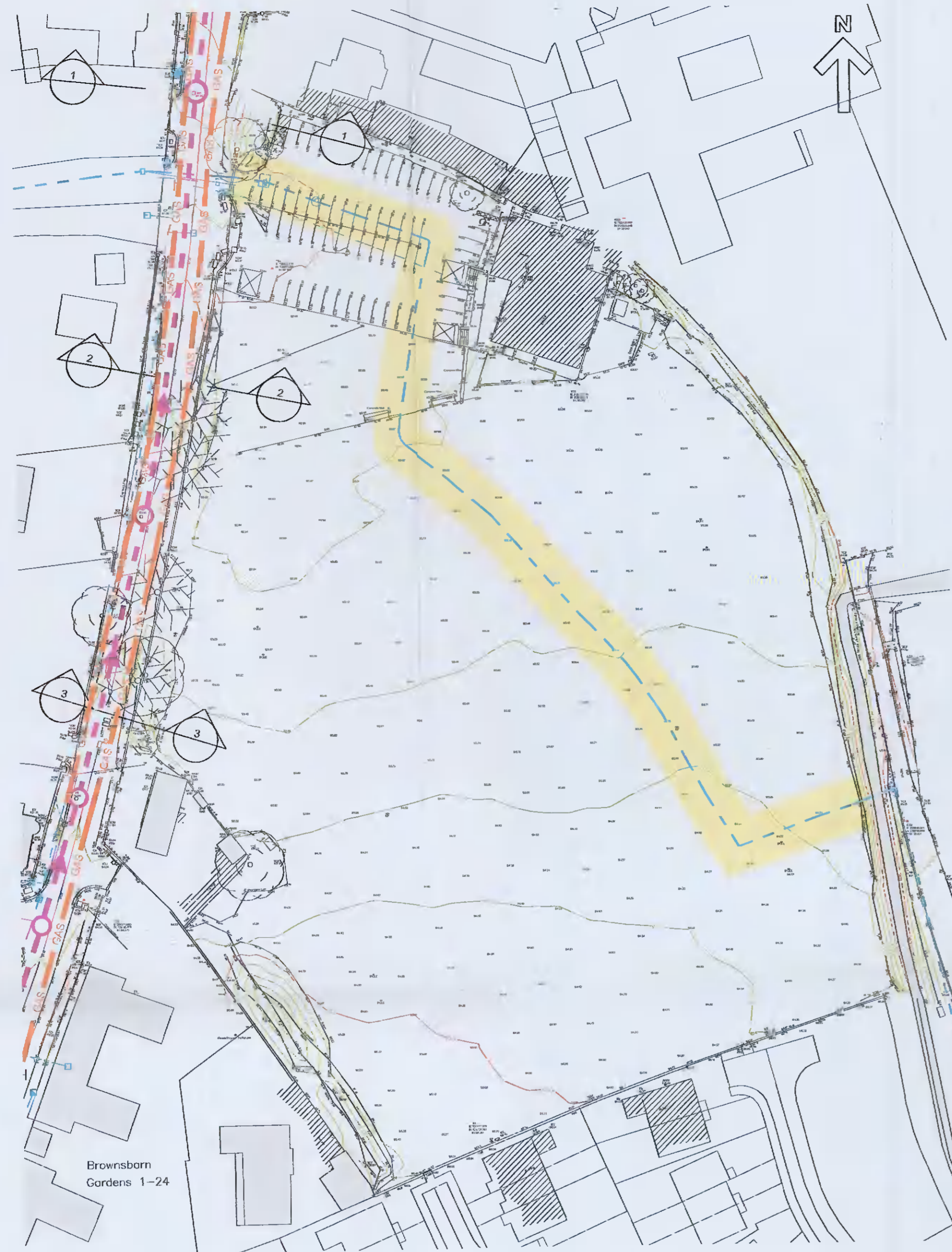
1 FOUL SEWER CONNECTION POINTS CONSIDERED SCALE: 1:750
