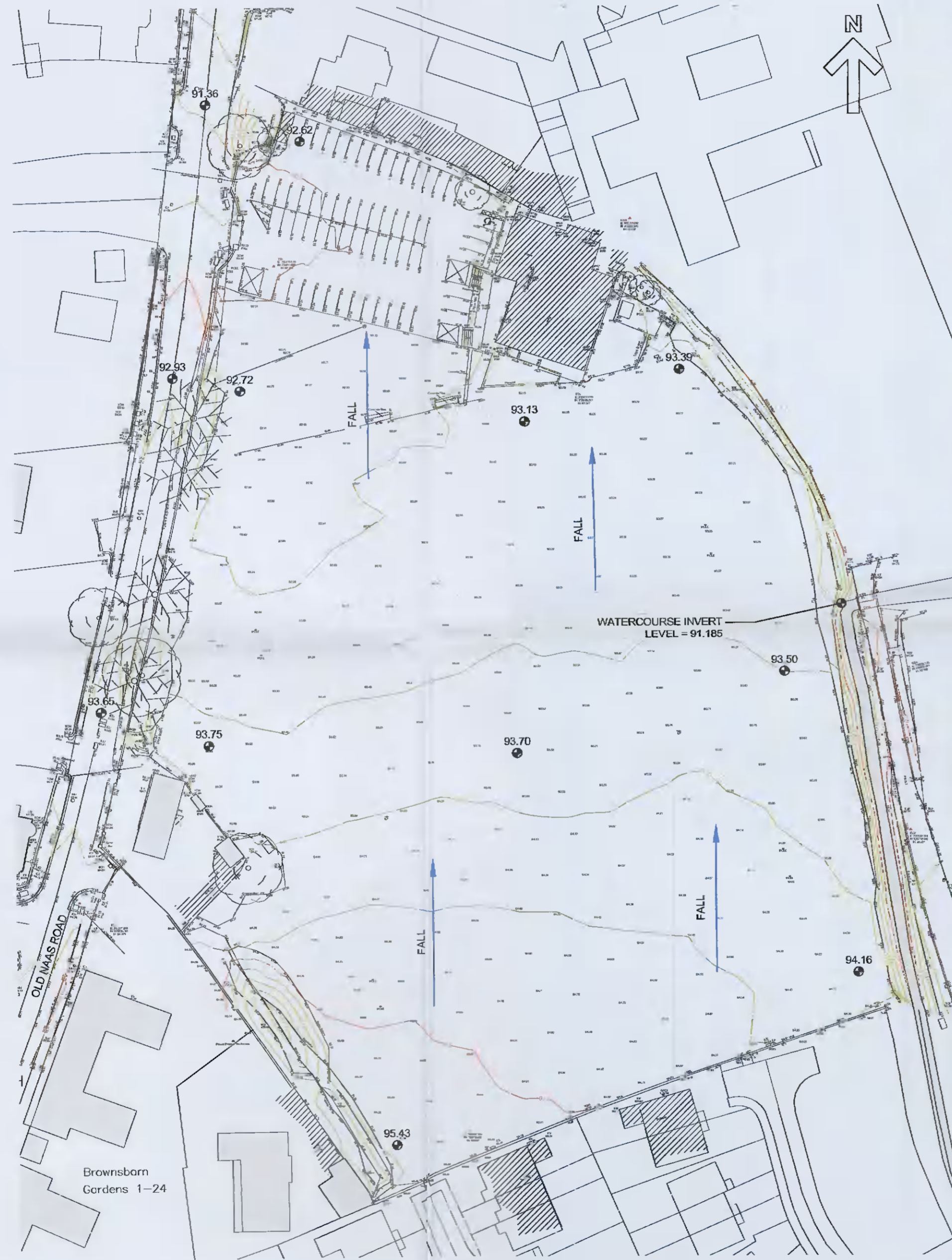
1 OVERVIEW OF EXISTING GROUND LEVELS SCALE: 1:750
