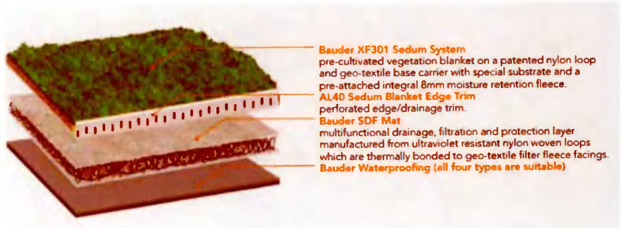
Figure 2 Extensive Green Roof
