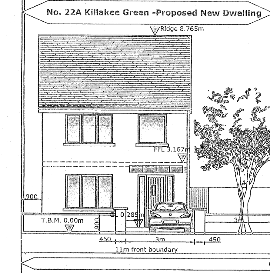
PROPOSED FRONT ELEVATION - BOUNDARY AND ENTRANCE GATE. 1:100
