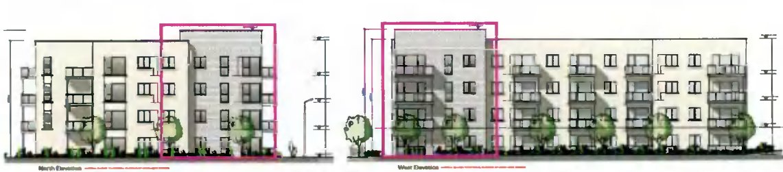
Figure 3: Extract from Drg. No. 2012 PA3 APT 05 prepared by Conroy Crowe Kelly Architects & Urban Designers denoting the proposed material changes to the North and West Elevations of Block 01 as highlighted in Figure 1.
