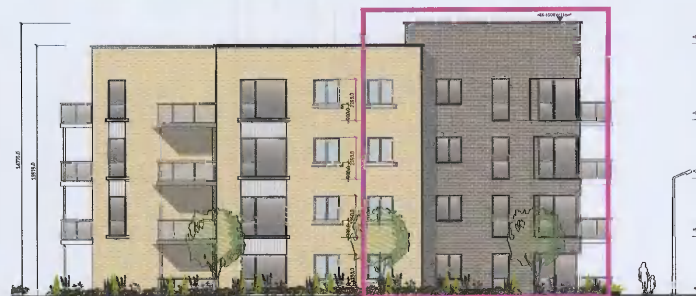
North Elevation MATERIAL CHANGE TO EXTERNAL CLADDING OF NORTH WEST CORNER
