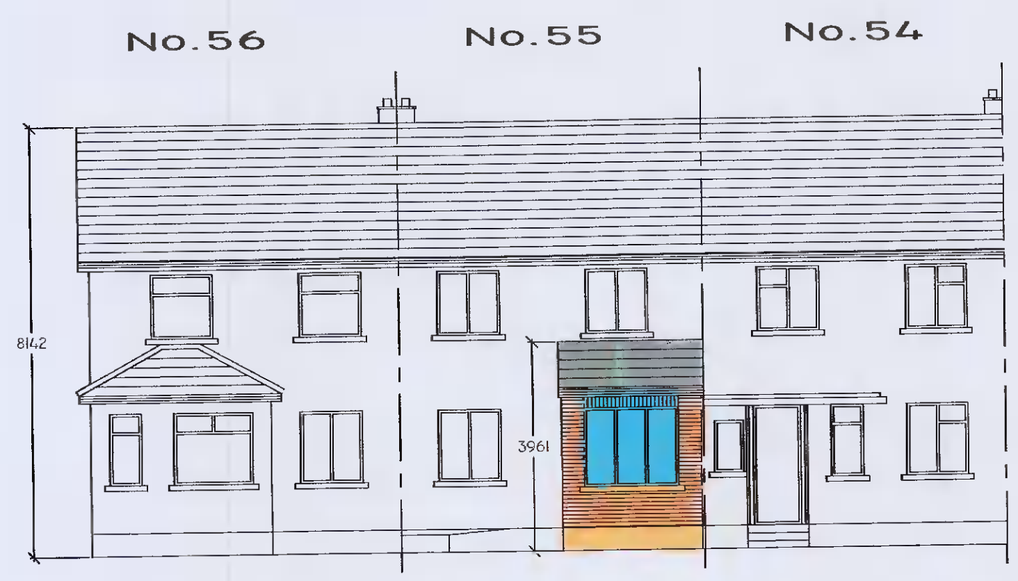
PROPOSED CONTIGUOUS FRONT ELEVATION SCALE: 1:100
