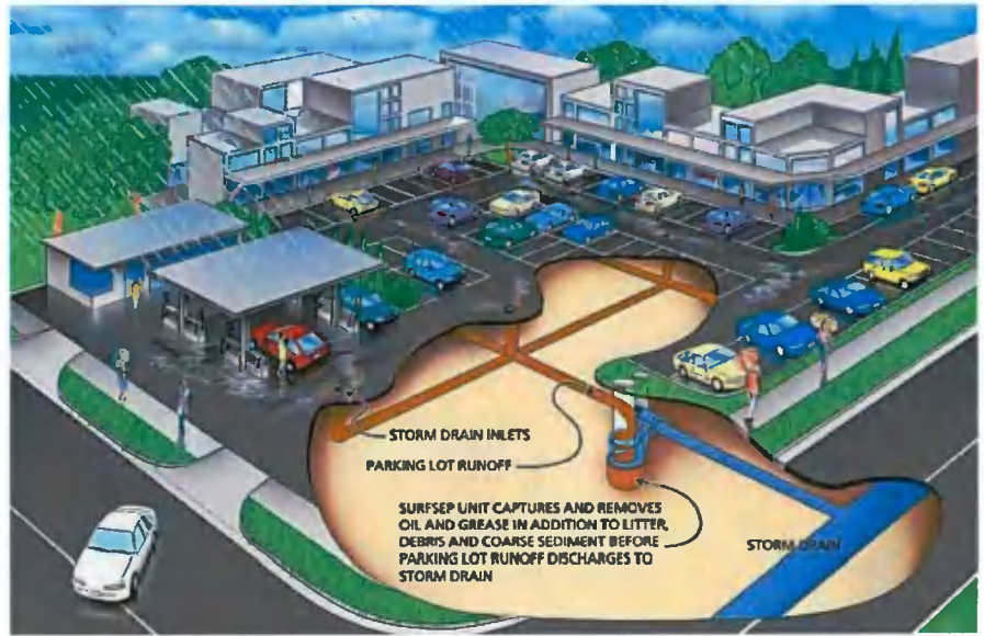
Typical SurfSep installation
