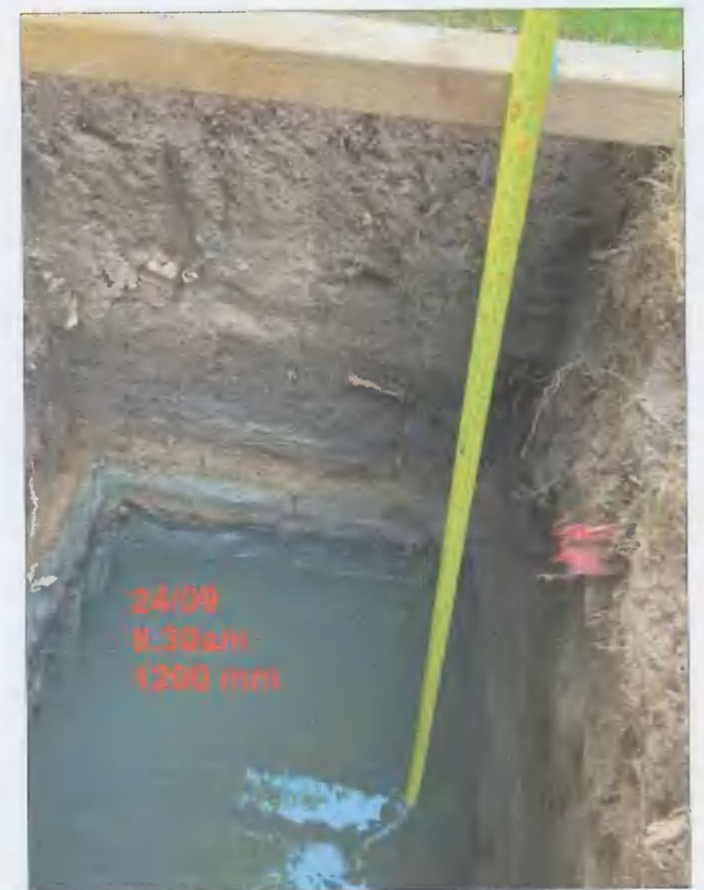
PERCOLATION TEST UNDERTAKEN 13-10-2021
