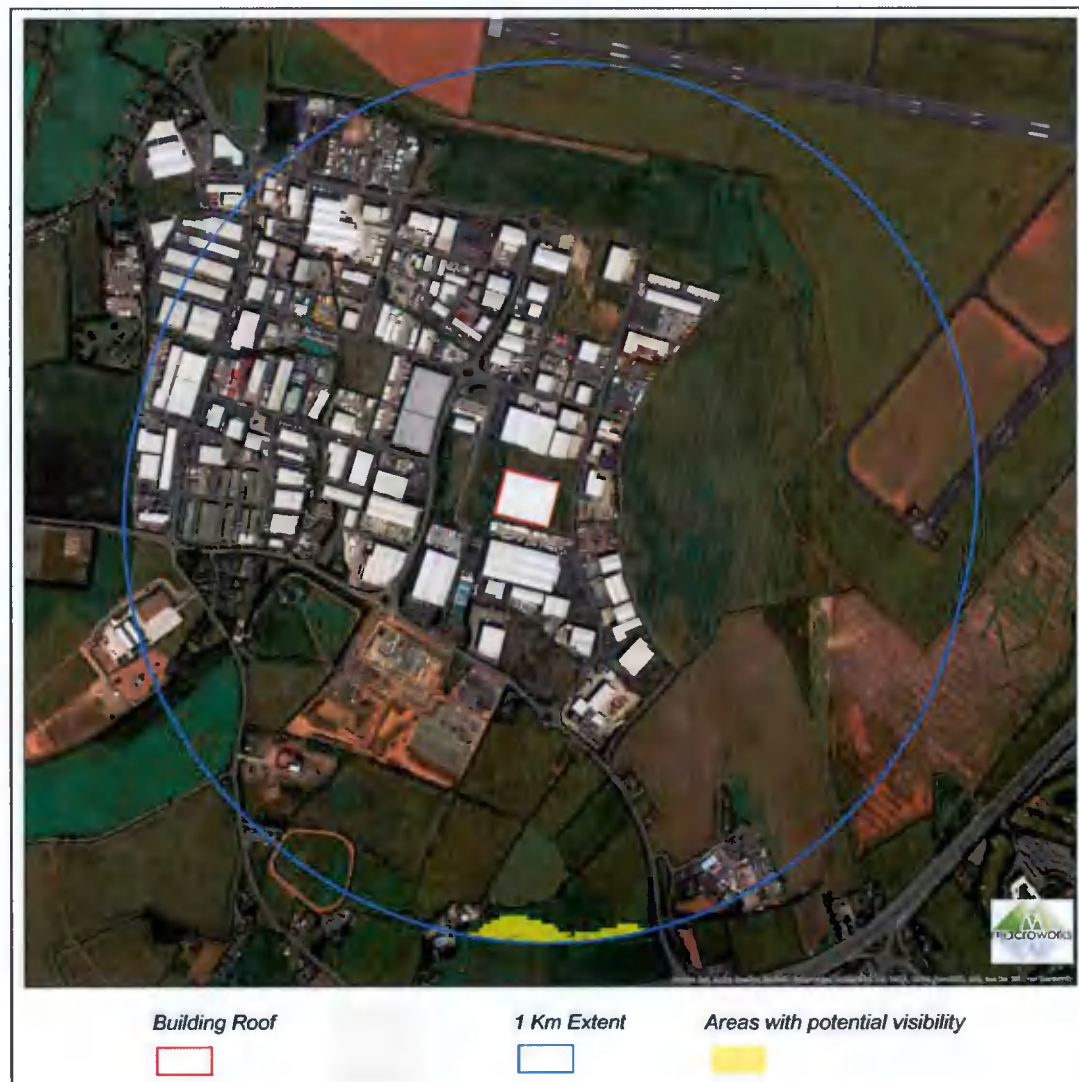
Figure 10: Parts of the study area it may be possible to see the proposed PV panels. The results are based on 3D terrain data that does not account for screening by vegetation or man-made structures. This is calculated for 1.7m above ground level which is indicative of eye-level of a person standing or a 4x4 vehicle driver.
